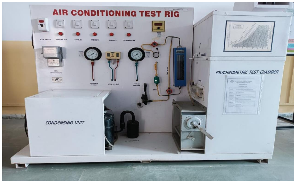
Figure 2. Photographic view of air conditioning test rig.
