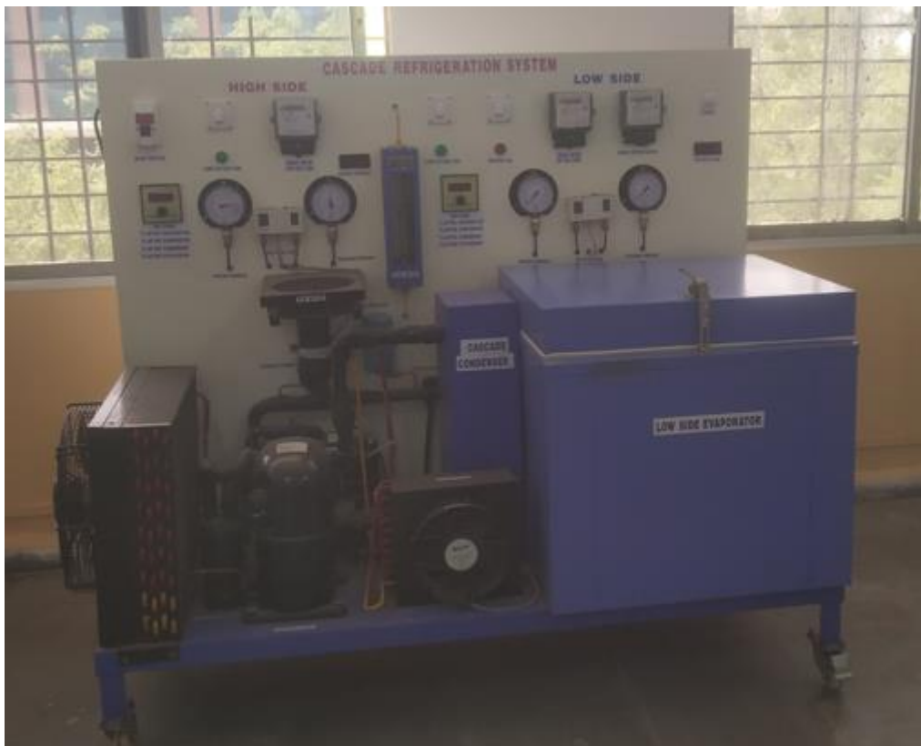
Figure2. Photographic view of cascade refrigeration system
