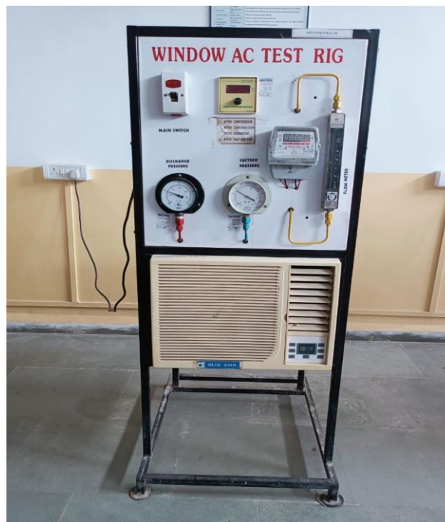
Figure2. Photographic view of window air conditioning system
