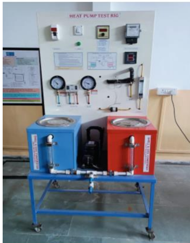
Figure 2: Photographic view of mechanical heat pump
