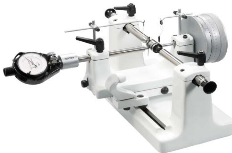
Fig.7.1 - Floating Carriage Micrometer
