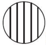
Fig 4.2 : Fringe pattern for flat surface
