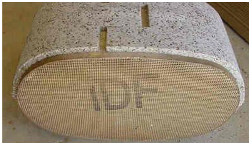
The ceramic honeycomb catalyst structure
