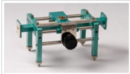
Figure 1.8. Slotted waveguide section
