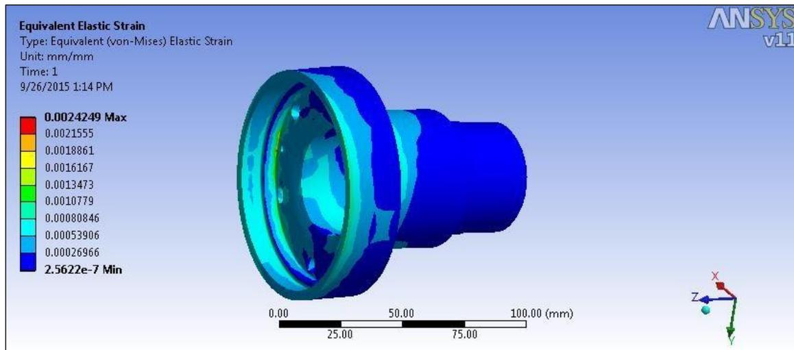
**Fig. 6:** Equivalent von-Mises Strain of SAE 1141 on 6800 N.
