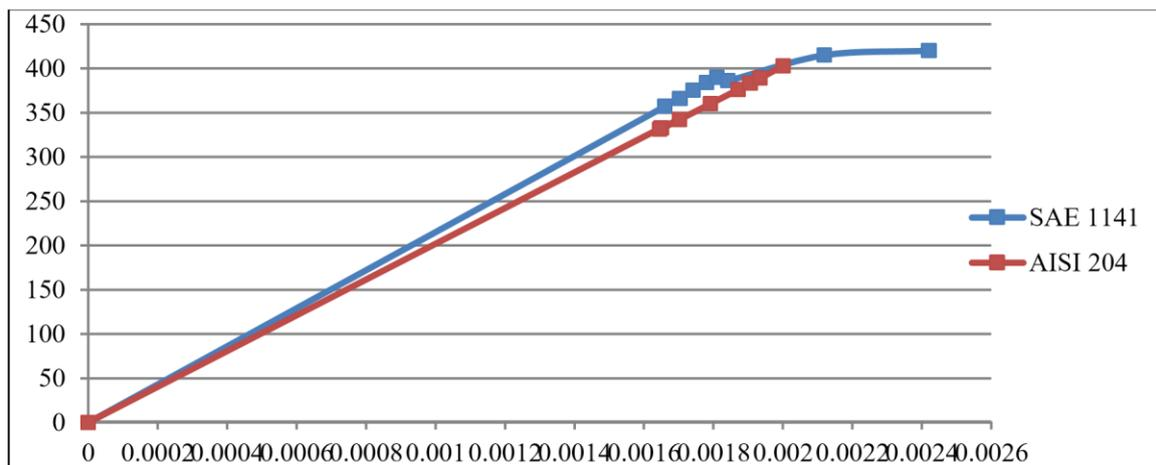
**Fig. 12:** Stress-Strain Curve of SAE 1141 and AISI 204 Companion Flange.
