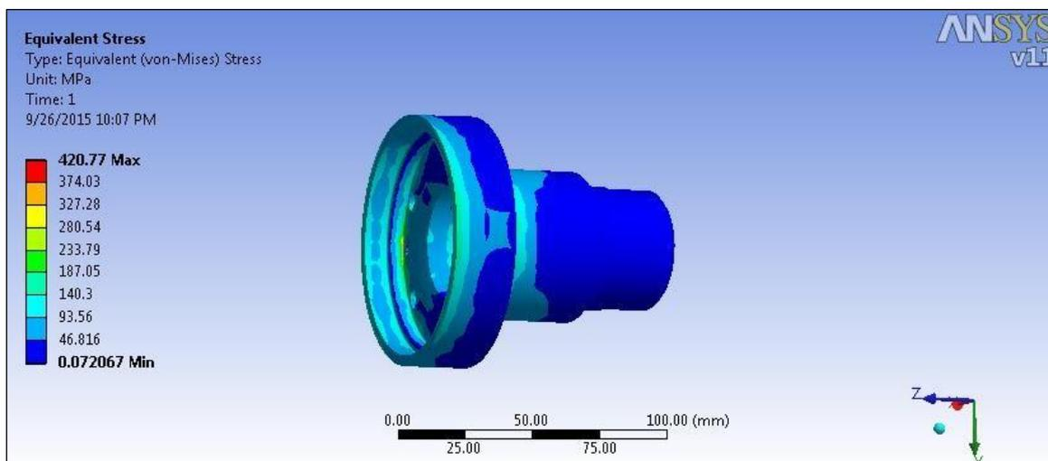
Fig. 5: Equivalent von-Mises Stress of SAE 1141 on 6800 N.
