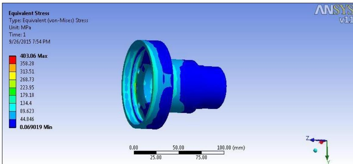
Fig. 8: Equivalent von-Mises Stress of AISI 204 on 6800 N.
