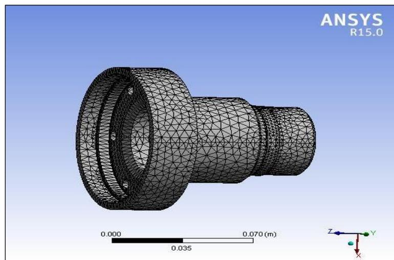
*Fig. 3: Finite Element Model.*
