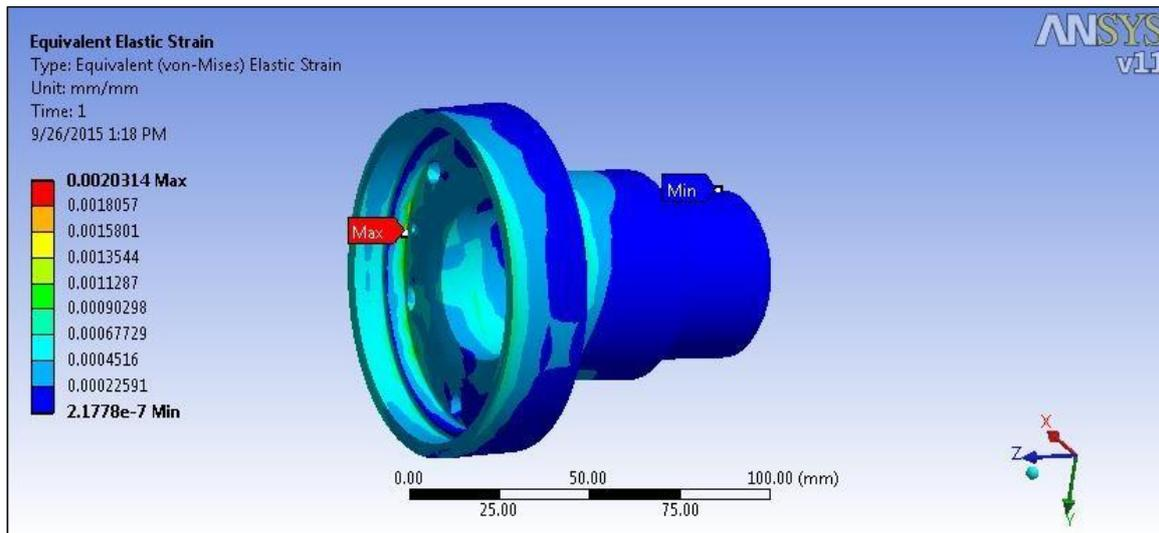
Fig. 9: Equivalent von-Mises Strain of AISI 204 on 6800 N.
