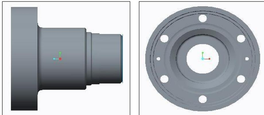
*Fig. 2: 3D Model of Companion Flange.*
