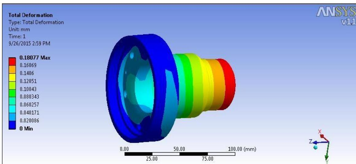
Fig. 10: Deformation of AISI on 6800 N.
