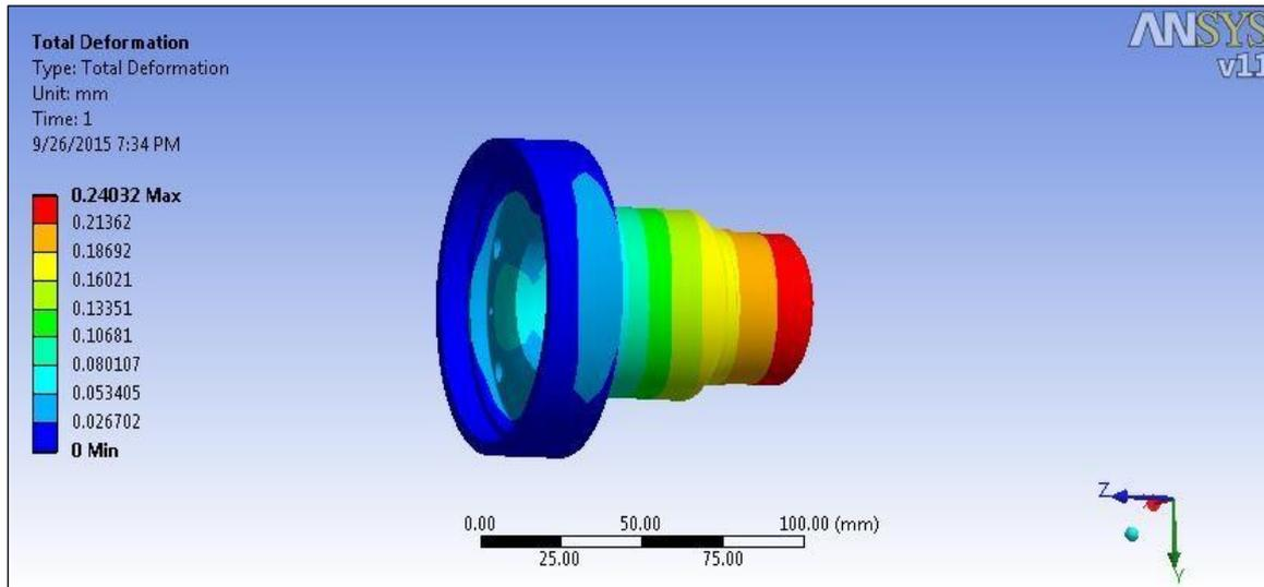
Fig. 7: Deformation of SAE on 6800 N.
