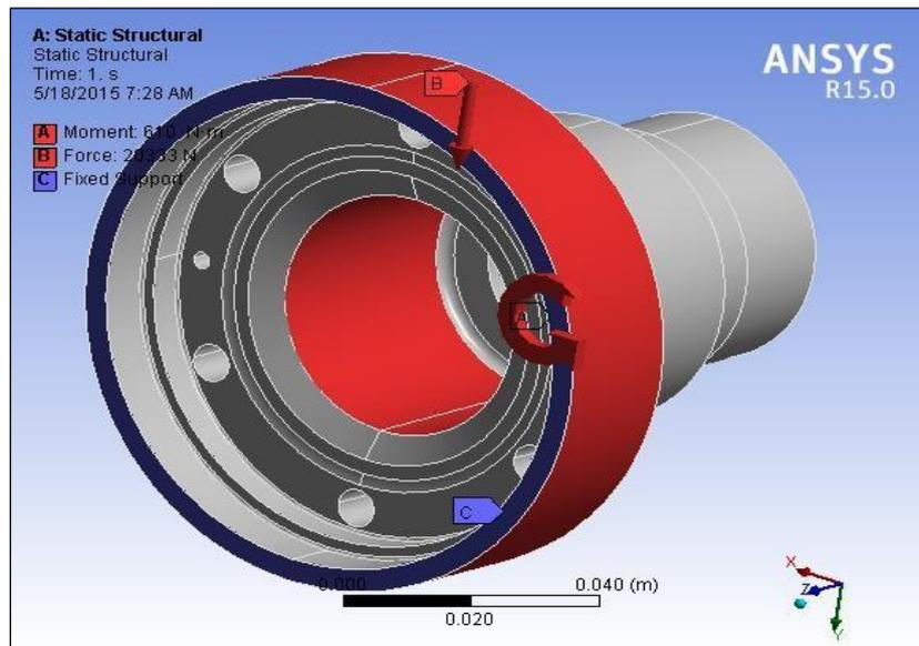
Fig. 4: Boundary Condition on Flange.
