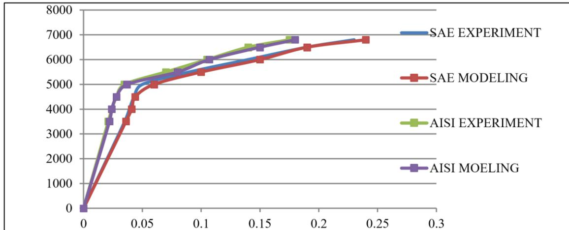
**Fig. 11:** Total Load-Displacement Curve of SAE 1141 and AISI 204 Companion Flange.
