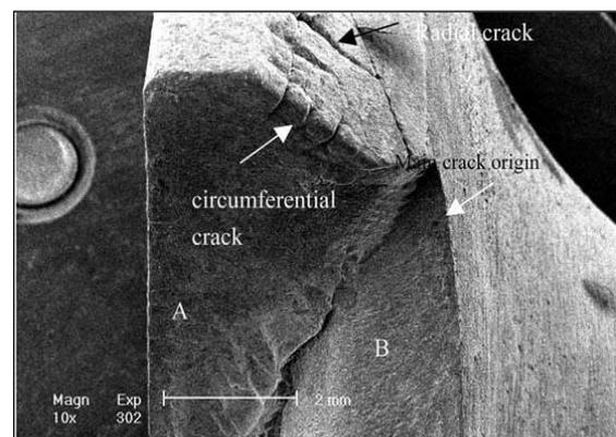
**Fig. 6:** SEM Image of the Fracture Surface of Valve no. 1.
