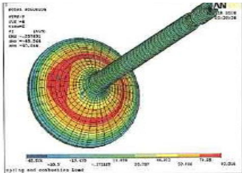
Fig. 4: Stress Analysis on Valve Neck under Spring Load [1].
