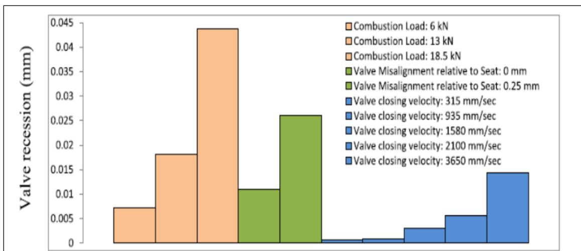
Fig. 2: Relation of Valve Recession [9].
