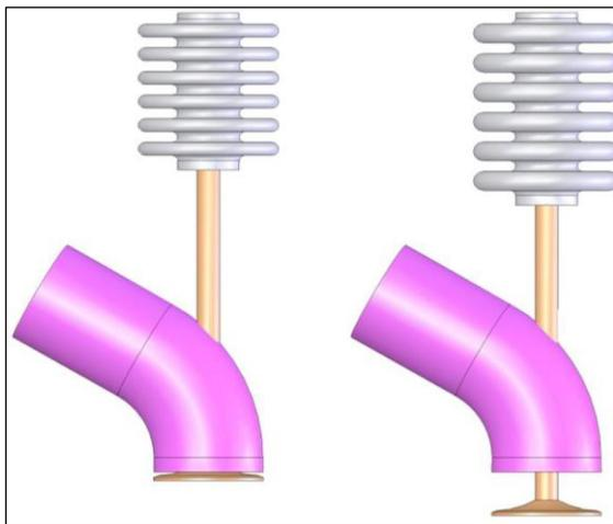
**Fig. 9:** Closed and Open Positions of Valve Actuated using Six Convolution Spring.
