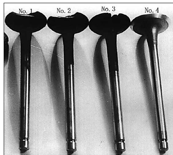
**Fig. 5:** Specimens of the Failed Valves no. (1,2,3) and New Valve (4).
