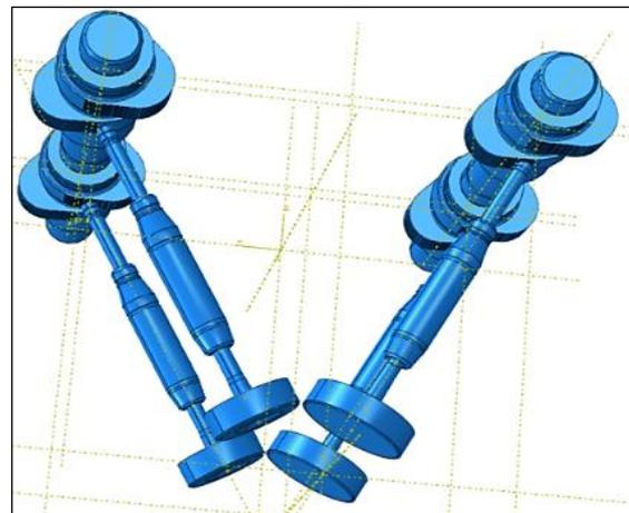
*Fig. 1: Finite Element Model of Valve-train*
