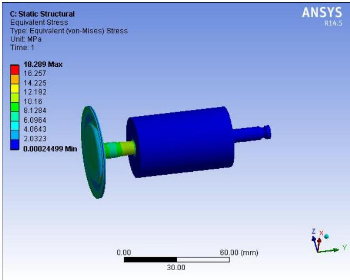
Fig. 7: Static Structural Analysis of Valve with Seat and Guide.
