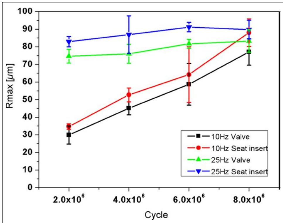
Fig. 6: Rmax and Rmax Rate of Valve and Seat Insert at 10 and 25 Hz.
